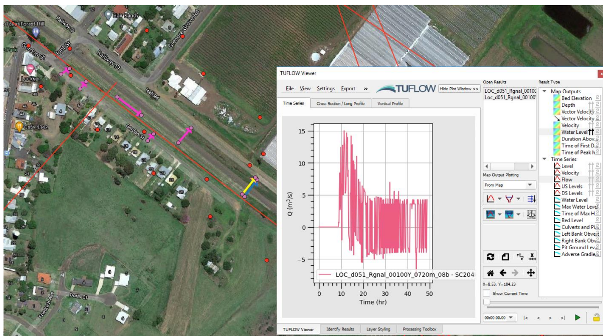
Figure 16: 1% AEP Developed Scenario Culvert Instability
