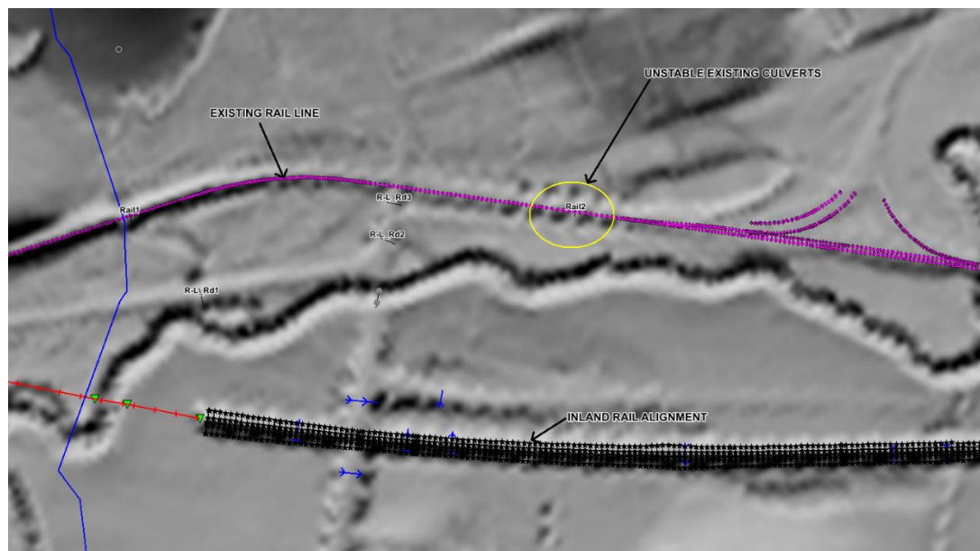
Figure 5: Location of Culvert with Model Instabilities
