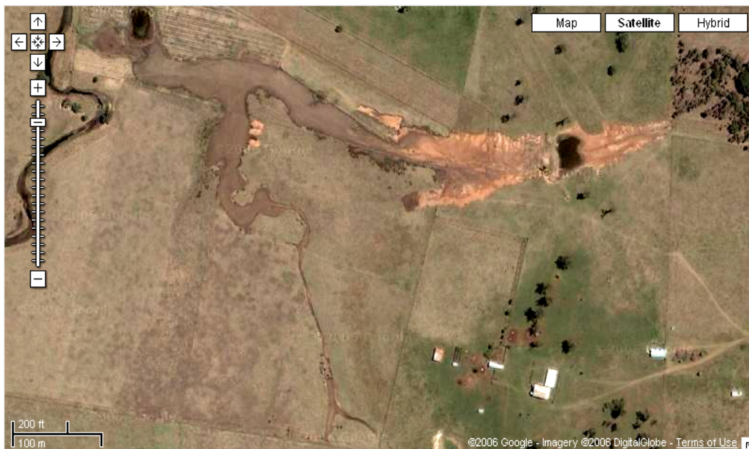
Figure 20. Example of the impact of a farm dam on salting in a drainage line in Winwill formation and the alluvium near Mt Tarampa in Plain Creek. The hydraulic barrier of the dam together with leakage has affected the upstream and downstream areas very significantly. Image from Google maps.
