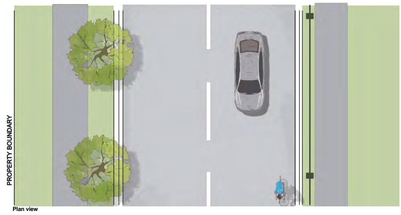
Figure 4.7.2 Collector road in urban setting, 2 lanes with cycle lane and paths between 2.0-2.5m wide - road corridor approx width 18-22m
